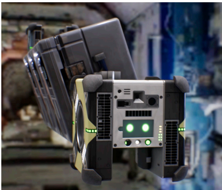
NASA expects that Astrobees, a free-flying robot, will begin working with humans aboard the International Space Station by the end of this year. This illustration shows what two Astrobees might look like as they cooperate to move cargo. Image courtesy of NASA.
